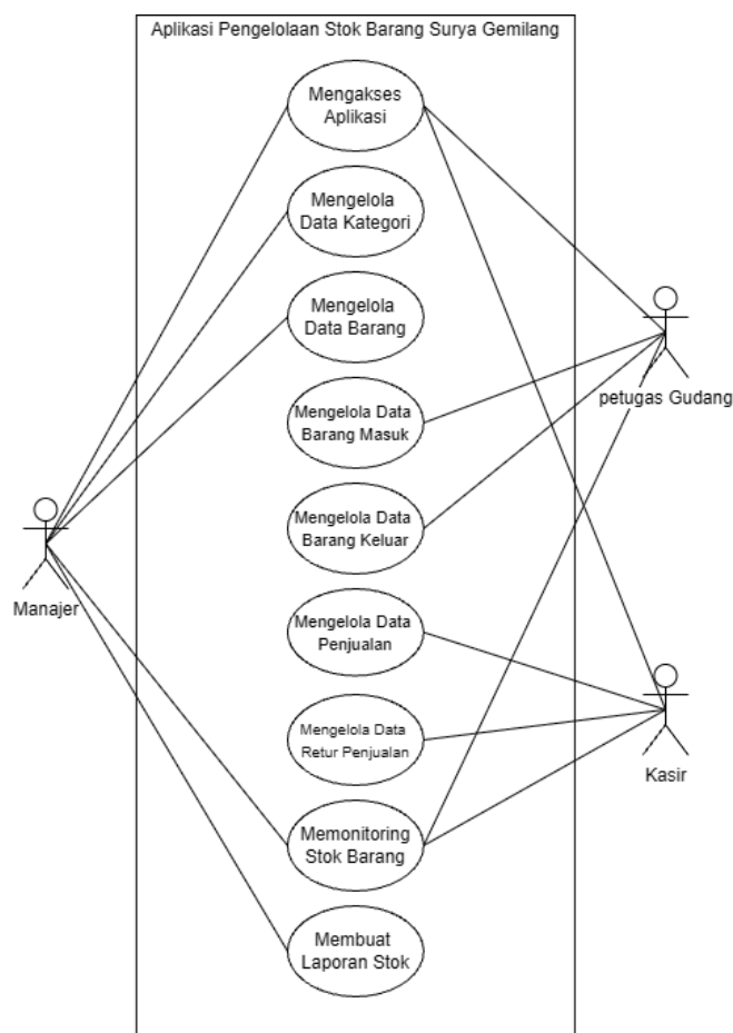
Gambar 4.6. Diagram Use Case Sistem Usulan
