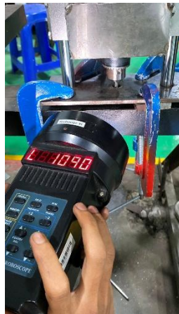
Gambar 22. Pengukuran putaran spindle saat proses friction welding berlangsung
