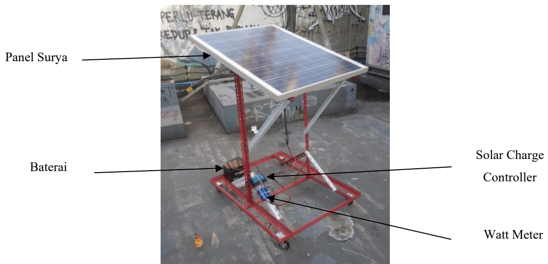
Gambar 26 Set Up Charging
