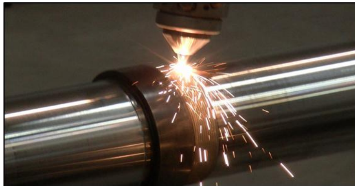
Gambar 5. Welding Overlay Cladding [18].
