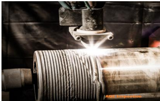
Gambar 1. Weld overlay cladding [5]
