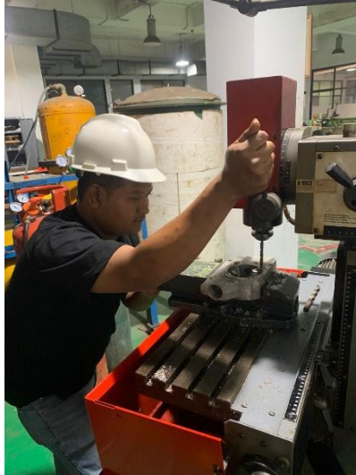
Gambar 22. Proses pengeboran samping kanan kiri gearbox
