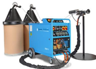
Gambar 31. Mesin metal coating
