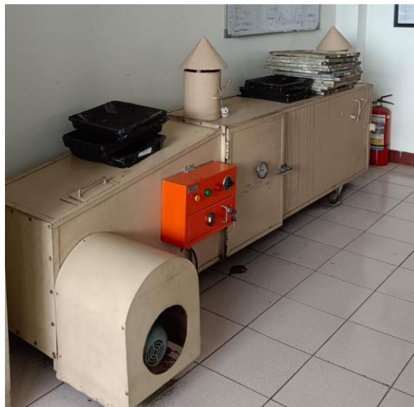
Gambar 5. Tunnel Dryer (Dokumentasi, 2025)
