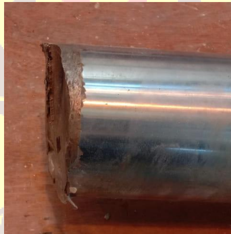
Gambar 11. Patahan Poros HWP
