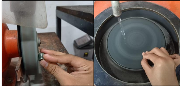
Gambar 28. a) proses grinding b) proses polishing
