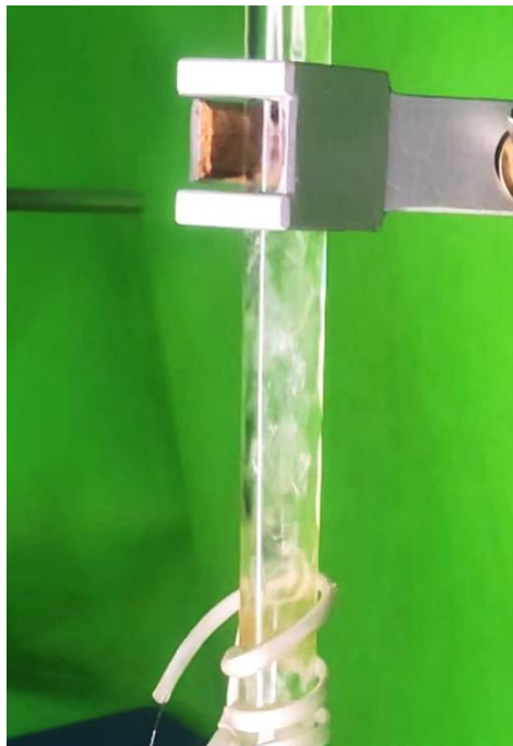
Gambar 4.44 Churn flow (70-110W)
