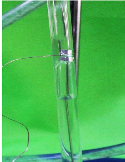
Gambar 4.48 Churn flow (30-50 W)
