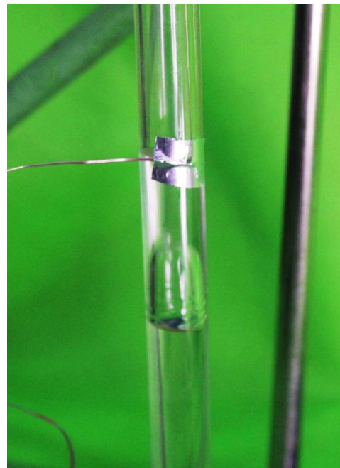
Gambar 4.24 Churn flow (30-50W)
