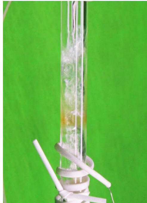
Gambar 4.9 Churn flow (50W)
