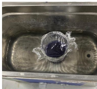
Ultrasonik t = 5 menit T = 30^{\circ}\text{C}
