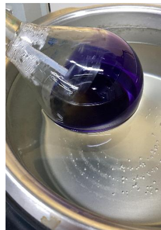
Evaporasi T = 50^{\circ}\text{C}
