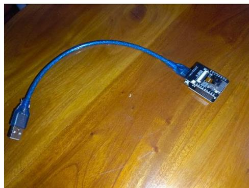
**Gambar 2. 2 Sensor Kamera Alat *Internet of Things* (IoT)**
