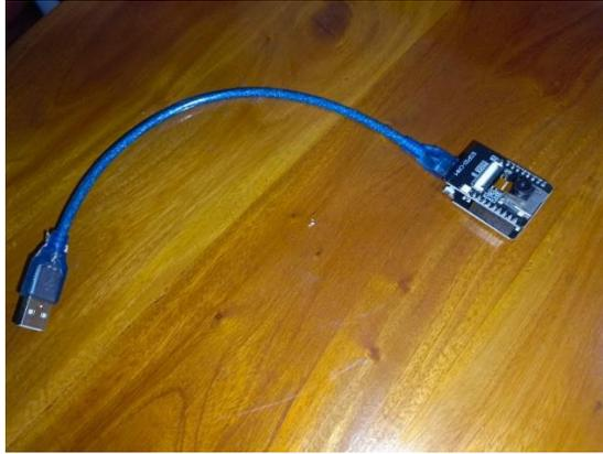
**Gambar 2.5 ESP32-CAM**
