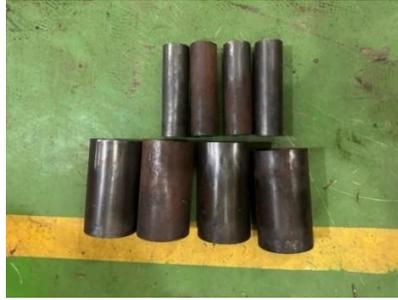
**Gambar 3. 12 Pipa Baja *Schedule* 40 Diameter 2 inch (50 mm) dan 4 inch (100 mm)**
