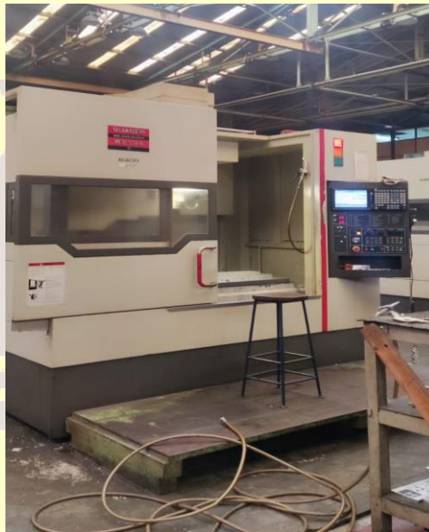
Gambar I. 1 Mesin CNC Milling MV184 (Sumber: Engineer PTDI )
