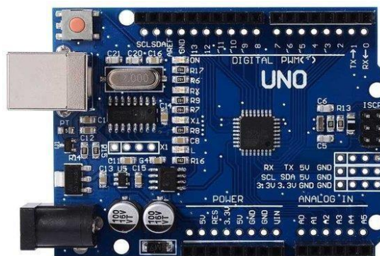
Gambar 12 Board Arduino UNO R3 [32]
