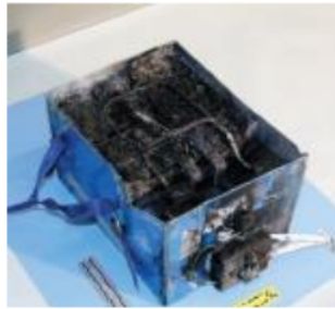
Figure 1. The burned and exploded Boeing 787 Dreamliner battery [1].
