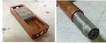
Fig. 4 Stainless steel screen mesh capillary wick
