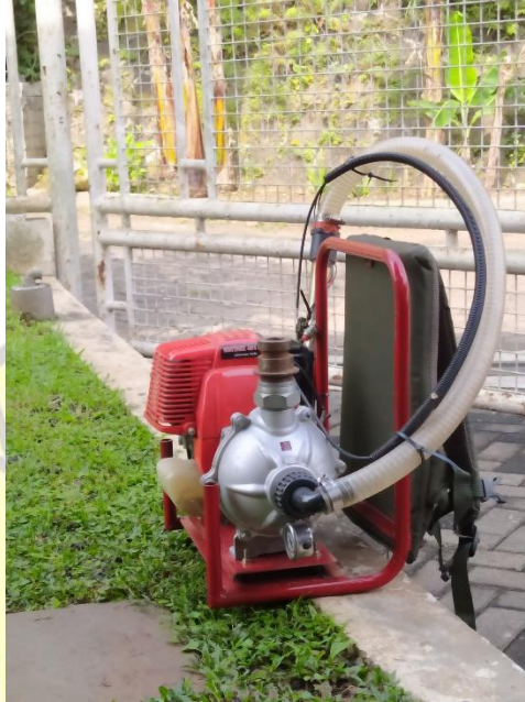
Gambar I. 2 Prototype Alat Fire Pump Portable
