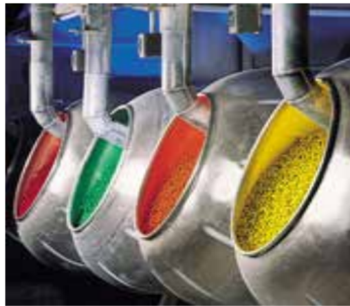
Gambar 5.3 Metode Pan Coating. (Sumber: tradeindia.com )
