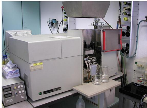
Gambar 2.6 Alat AAS (*Atomic Absorption Spectrophotometry*)
