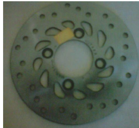
Fig 4. Ventilating Holes 8 mm
