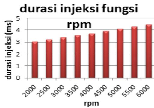
Gambar 2. Mapping durasi injeksi fungsi putaran engine
