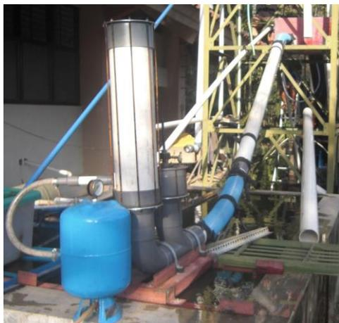
Gambar 1. Instalasi Pompa Hidram
