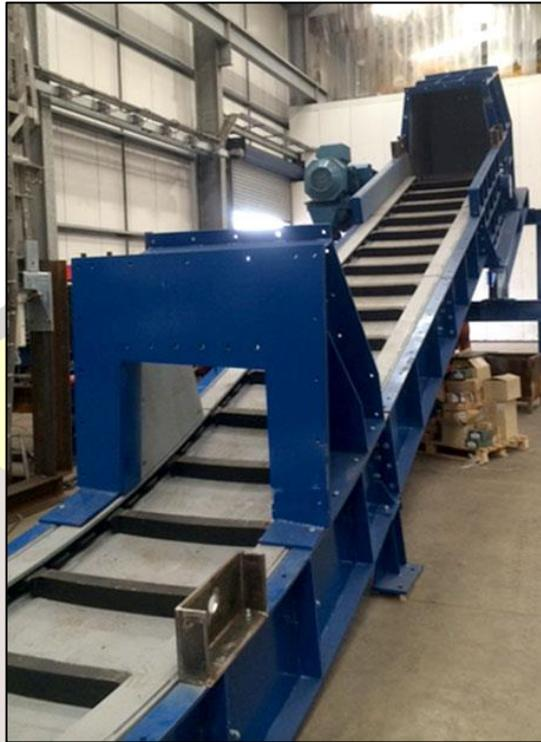
Gambar 2.2 *Scraper* Konveyor
