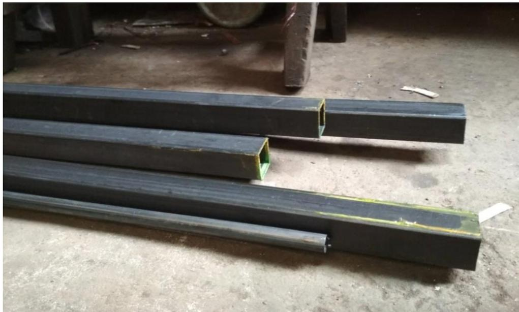
**Gambar 4.3** Material Awal Rangka Konveyor
