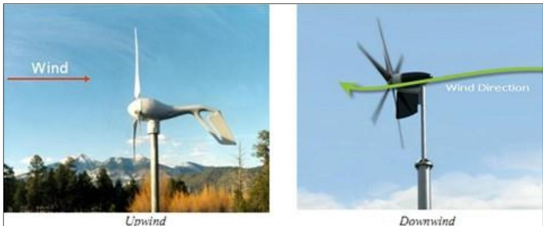
Gambar 2.5 Turbin angin jenis *upwind* dan *downwind*
