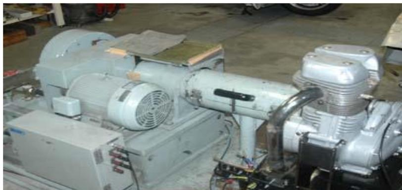
**Gambar 2.52** Dynamometer Engine
