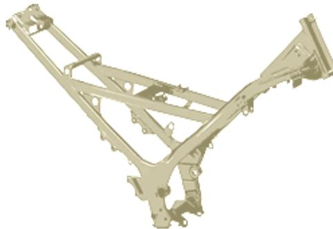
**Gambar 2.46** *Rangka Tipe Underbone*
