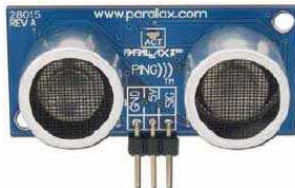
Gambar 2.6 Ping))) Parallax Ultrasonic Range Finder
