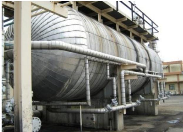
**Gambar 2.4. Pressure Vessel**
