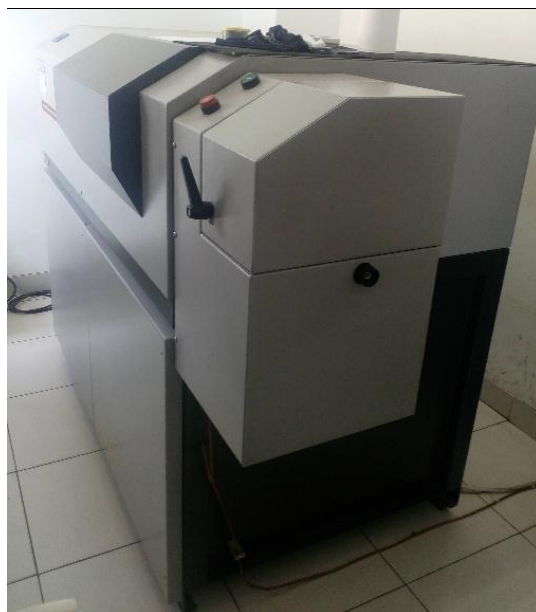
Gambar 3.3 ARL 3460 Optical Emission Spectrometer .
