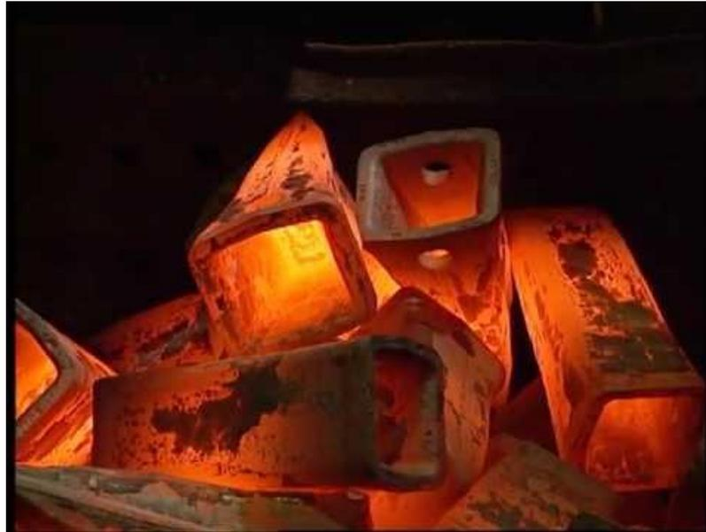
Gambar 2.14 Hasil pengecoran *Bucket teeth* <sup>[5]</sup>
