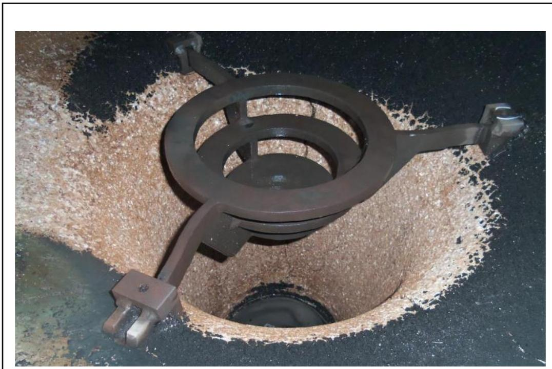
Gambar 2.5 Current Design Erosion Protection Shield
