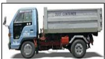
c. *Arm-roll truck, Roll-on truck, Multi-loader truck*
