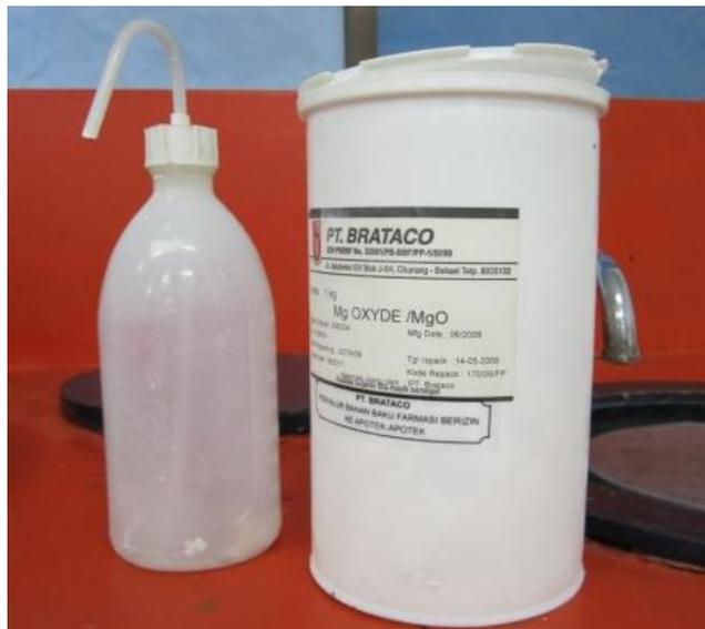
Gambar 3.12 Pasta *Magnesium Oxide* (MgO)
