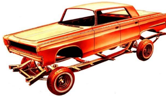
Gambar 2. 5 Body on frame.
