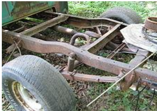
Gambar 2. 4 frame of 1956 chevrolet 1/2 ton. Shaped crossmember in background, c shaped rails and crossmember in center, and a slight arch over the axle
